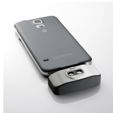
Figure 31.3 2015: FLIR One, an accessory to iPhone and Android mobile phones. Weight: 90 g (3.2 oz.).
