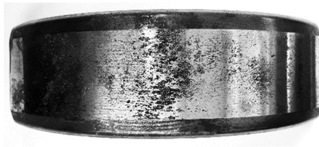
Figure 2. Material fatigue of a rolling bearing.
