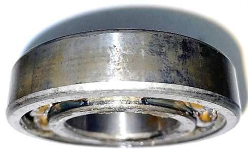
Figure 3. Corroded surface of a rolling bearing.
