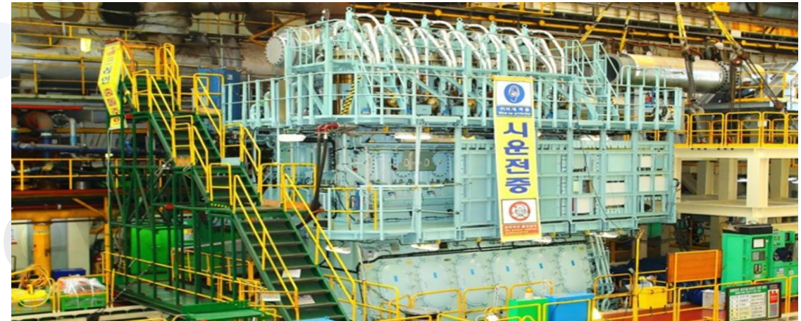
LPG Fuelled 2 – Stroke Engine on Test Bed
