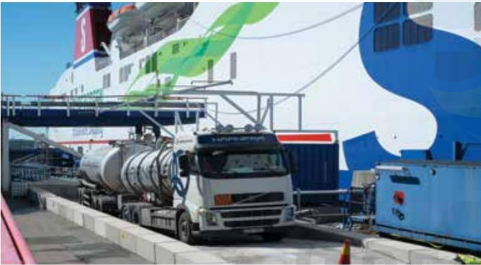
Stena Germanica methanol bunkering, Gothenburg
