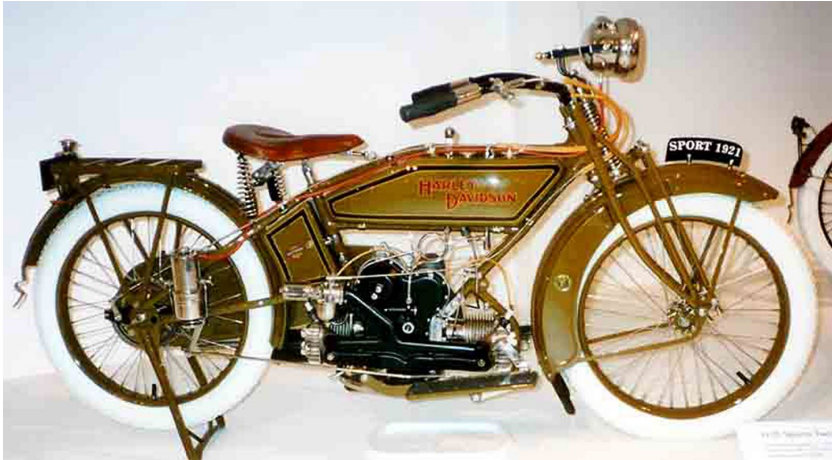
Figure 66: A Harley Davidson Sport 558 cc from 1921 displaying a stressed member engine where the tubes of the chassis are bolted directly to the engine, and the engine completes the structural triangle of the frame (By Lars-Göran Lindgren Sweden Wikimedia Commons).
